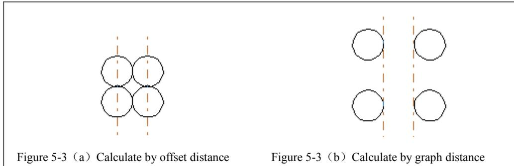
**Calculate by graph distance:** The space of the graphs is calculated by graph distance.
