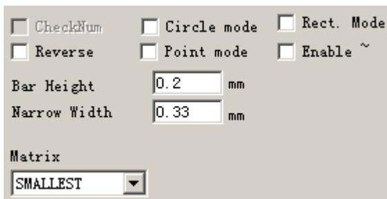
Figure 4-21 Data Matrix Barcode Parameter Setting
